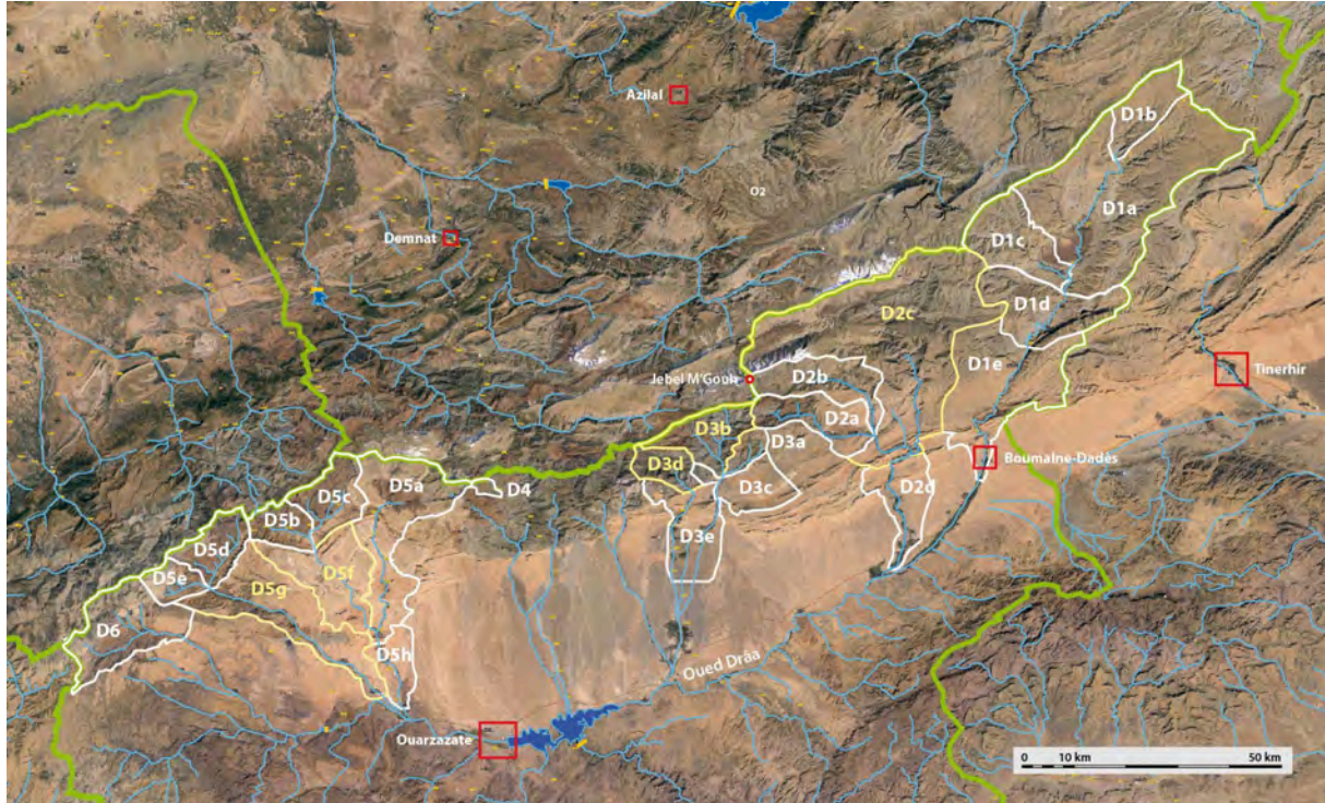
Fig. 367: Satellite image of potential study areas on the southern slope of the High Atlas Mts. in the upper Oued Drâa catchment. Streams and rivers are light blue, watersheds are light green. Boundaries of well documented study areas are white. Boundaries of areas with insufficient documentation are yellow. These areas, however, are similar to well known neighbouring areas.
