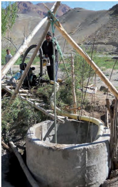
Well with a mobile motor pump, used for irrigation of apple trees near Outerbate, High Atlas.
